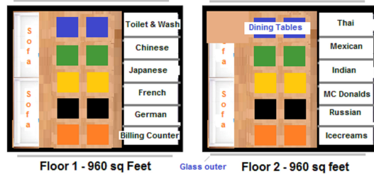
6 * 20 Feet Containers modified into 960 Feet Rooms
